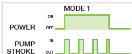
Figure 53: Mode 1 timing diagram
