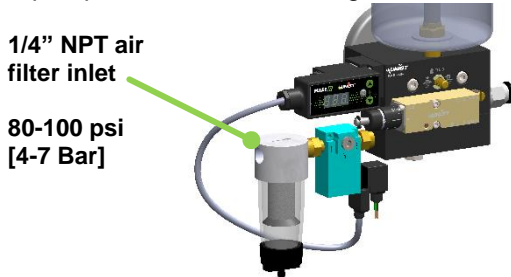
Figure 21: Air supply to filter
